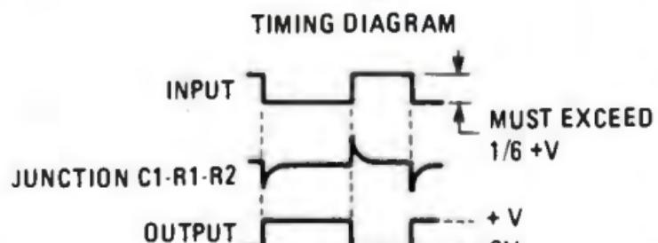
\*TIME CONSTANT  $RC < 10\mu s$  ( $C = C_1$ ;  $R = R_1 \parallel R_2$ )
